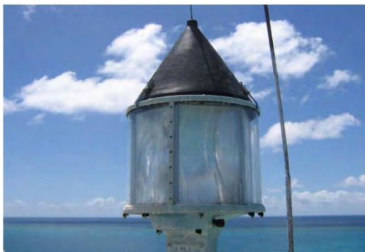
Figure 2. Adding cones to flat lantern surfaces
